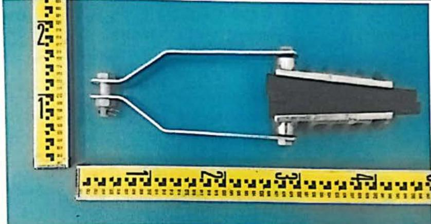
A photograph of an NXJG-4 insulator clamp. The clamp is a metal component with two curved arms on the left side and a central mounting point on the right. It is placed against a blue background. A yellow ruler is positioned vertically on the left side of the clamp, showing a scale from 0 to 20 centimeters. Another yellow ruler is positioned horizontally below the clamp, also showing a scale from 0 to 20 centimeters. The clamp's length is approximately 15 centimeters. | —  |
